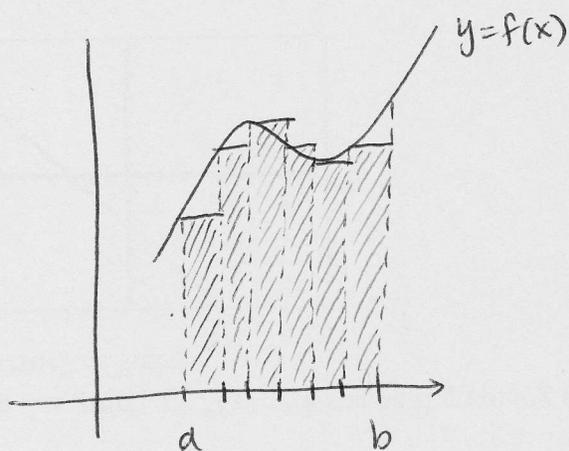
function height at left endpoint of each subinterval.
